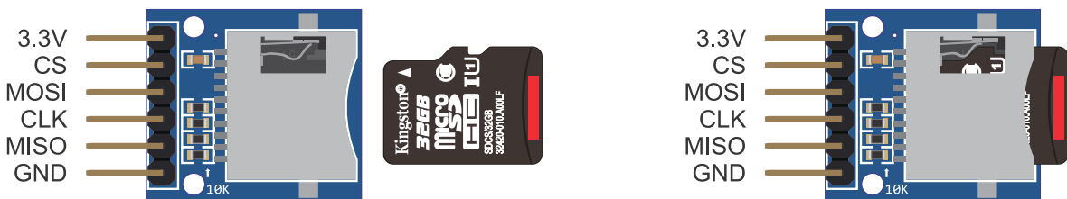
Figure 9.3 Details of the SD card module pins and how to insert the SD card into the module.
