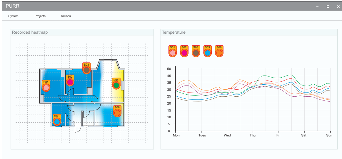
Figure 11.21 Example of an Mbed-based system having a web service with real-time insights, alerts and reports.
