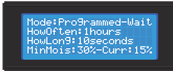
Figure 12.8 Layout of the LCD for the Programmed irrigation mode when the system is waiting to irrigate.
