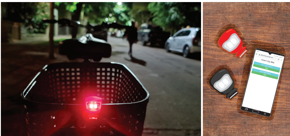
Figure 8.17 On the left, smart city bike light mounted on a bike. On the right, rear and front lights and the mobile app.
