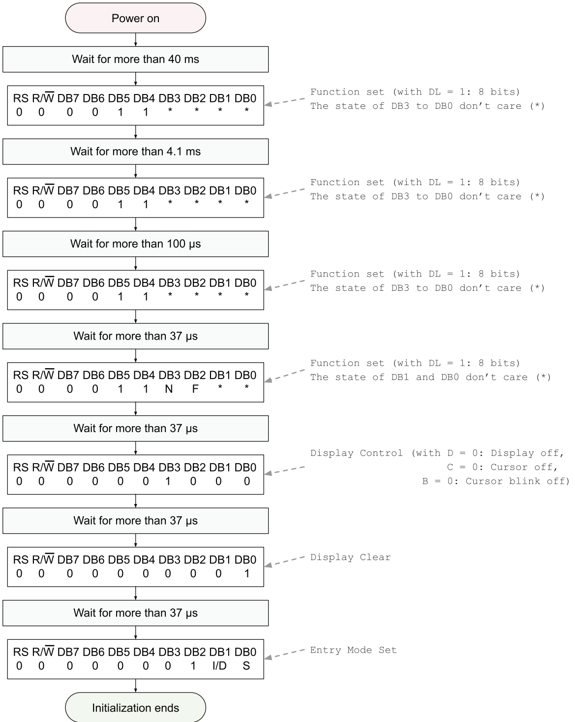
Figure 6.11 Initialization procedure of the graphic display when an 8-bit interface is used.
