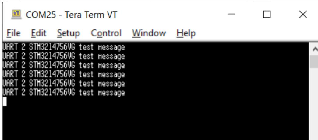
**Step 6:** Change the UART2\_TX pin to 'PA2' and generate the code and run the project. Attach logic analyzer 'D0' to pin 'PA2' and GND to GND pins. Click on 'Add protocol decoder' and from 'decoder selector' window double click on 'UART' protocol.
