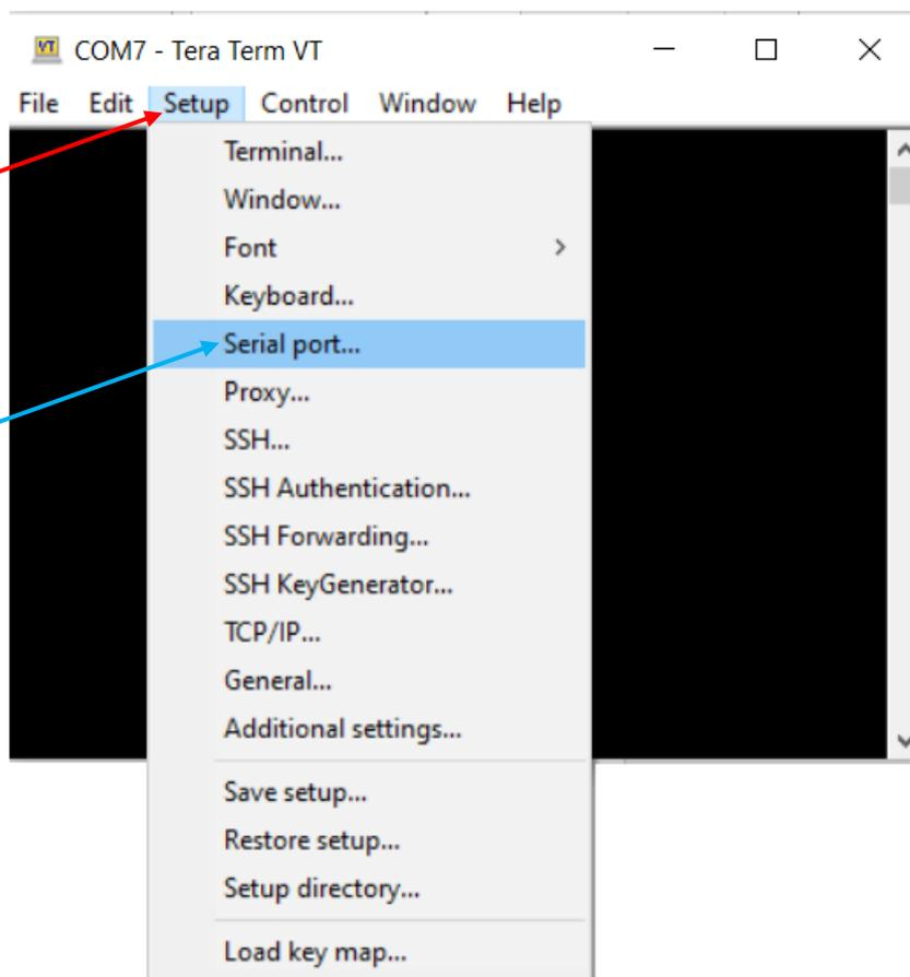
Configure the speed to '115200' and verify the other parameters to STM32L4 UART parameters and finally click on 'New Setting'.
