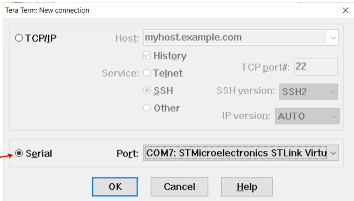
In TeraTerminal software click on Menu 'Setup' and select 'Serial Port'.
