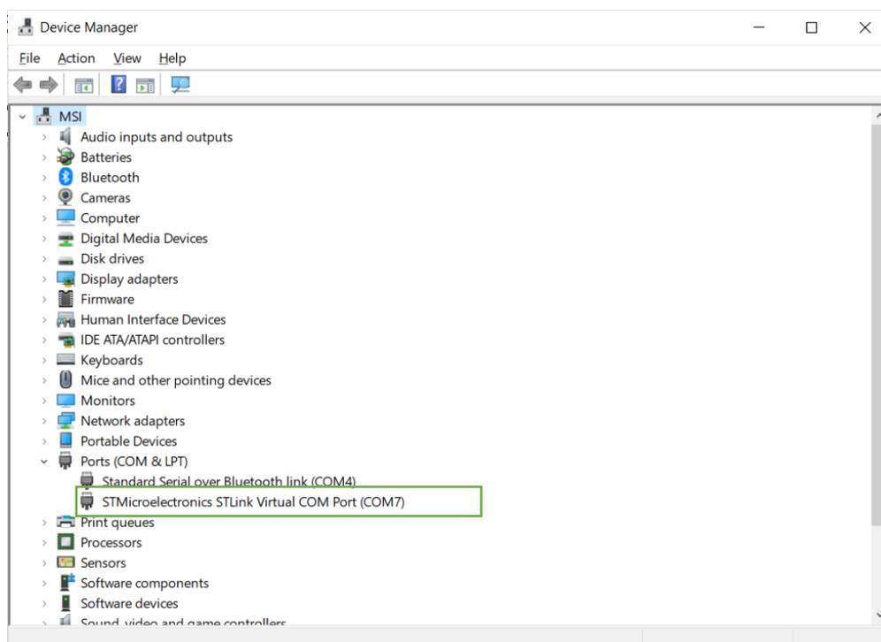
**Step 5:** [Install](#) and Open 'TeraTerminal' software and select the 'Serial' option and in port menu select 'STMicroelectronics STLink Virtual COM Port'.
